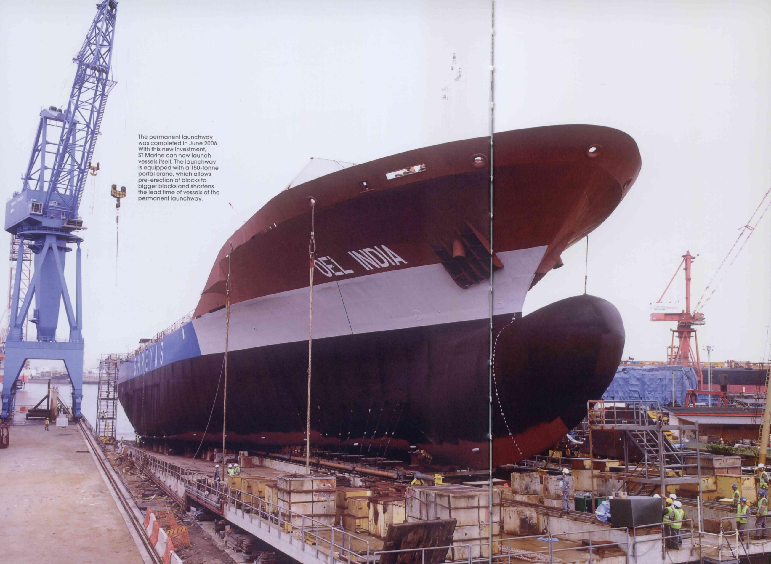
The permanent launchway was completed in June 2006. With this new investment, ST Marine can now launch vessels itself. The launchway is equipped with a 150-tonne portal crane, which allows pre-erection of blocks to bigger blocks and shortens the lead time of vessels at the permanent launchway.
