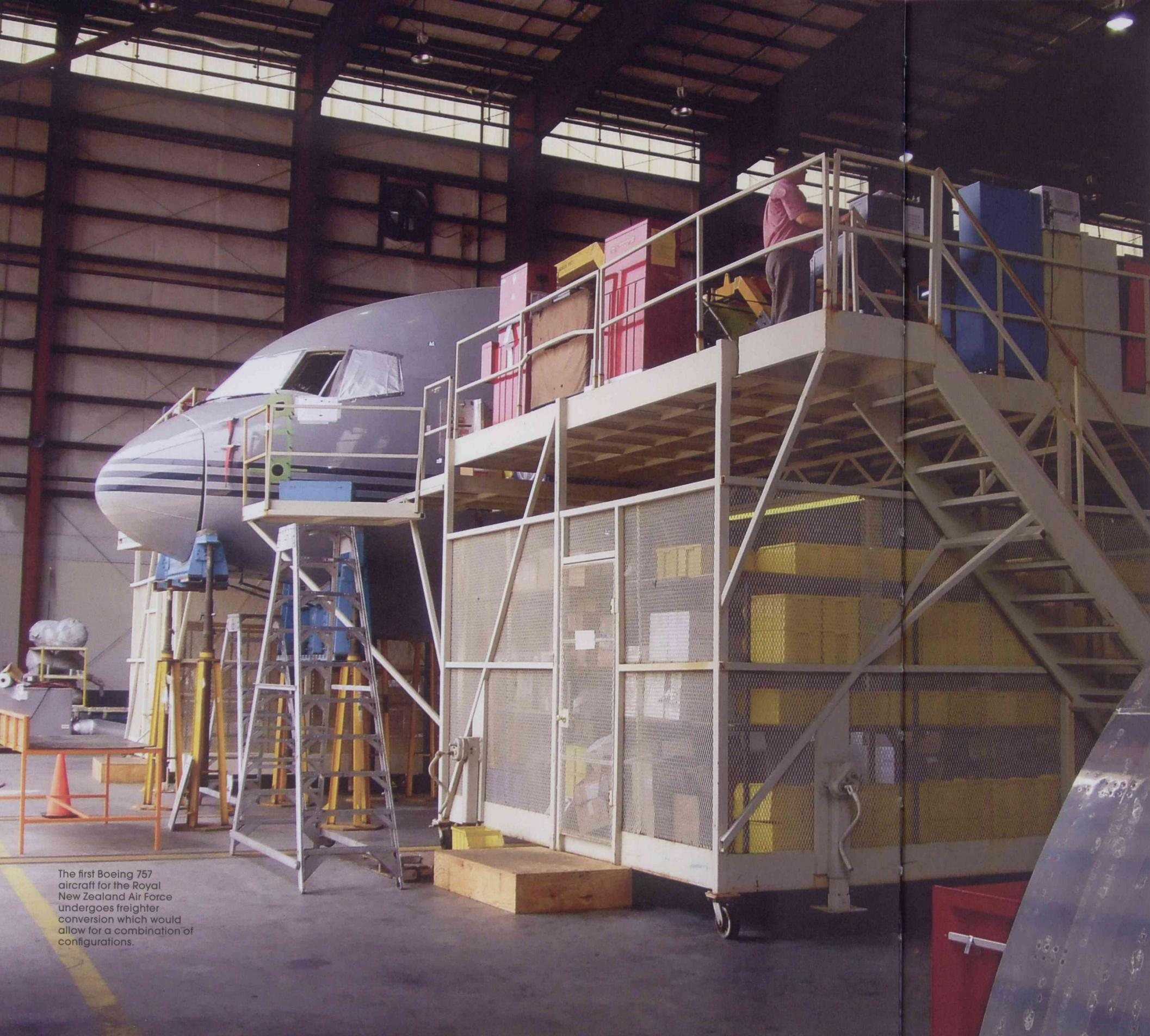
The first Boeing 757 aircraft for the Royal New Zealand Air Force undergoes freighter conversion which would allow for a combination of configurations.
